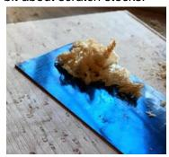
Just a small sample of the fine shavings you can get from using a scrapper vs. sandpaper to finish a project.
